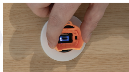
Insert the second part of the TUF Replacement tool until a click is heard (4 clips engage in TUF cartridge)
